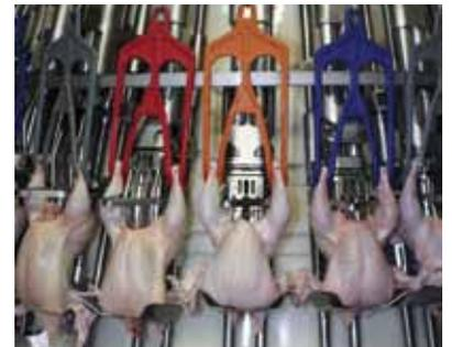
Setting a new standard in carcass cleanliness, the brand-new Marel Stork Poultry Processing final inspection machine, the FIM 20 Rotovac RS (Reference Series), achieves its results with little to no rib or carcass damage.
