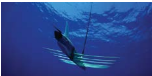
Subsea view of the Wave Glider with the Float on the surface of the ocean (top) and the Sub (center), 8 meters below. (Photo courtesy of Liquid Robotics, A Boeing Company)
