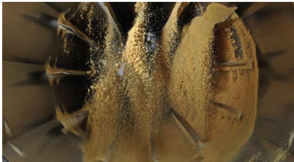
JAINDL BIOFUEL PLANT DRUM COOLER: The drum cooler can cool the soybean meal from 350 down to 75 degrees at the rate of 10 to 12 tons per hour.
