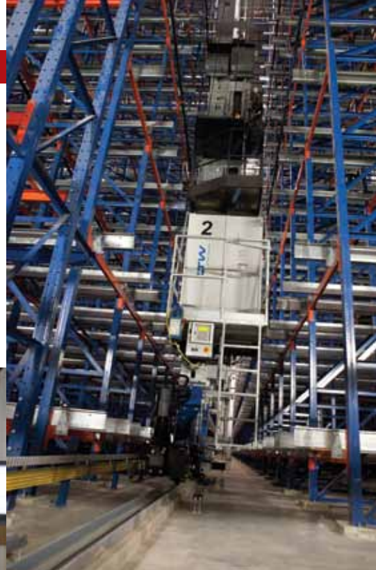
Preferred's opening celebration gave guests a first-hand look at how curve-going, rail-guided robotic stacker cranes can precisely handle pallet loads of goods in complete darkness. The new facility encompasses more than 10 million cubic feet combining precision automation with rapid product transfer.
